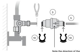
pressure reducer! The arrow should be pointing towards the A2O Pure (away from the inlet water ball valve).
